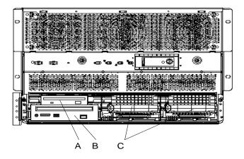
Figure 3-7: Chassis Drive Bays
